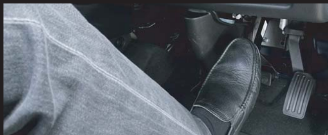
The driver releases his/her foot from the brake pedal. The car remain at a standstill for a maximum of two seconds
